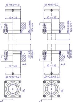
\* Note: for the FCSC flange, upside down installation is OK for all stroke lengths
