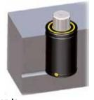
**Drop-In** The gas spring is dropped into a flat bottomed pocket within the die.
