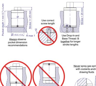
Never mount a gas spring in a pocket that does not fully support its base Never mount a gas spring in a pocket upside down
