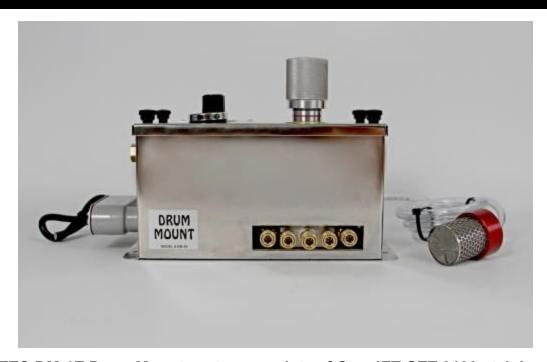
The JET-SET® DM-1E Drum Mount system consists of One JET-SET 9100 stainless steel piston pump (0-5cc per stroke) with 5 outlets for spray nozzles. The 9100 pump is engaged using the electric solenoid to receive external signals for system activation. The DM-1E comes standard 110v unless specified.
