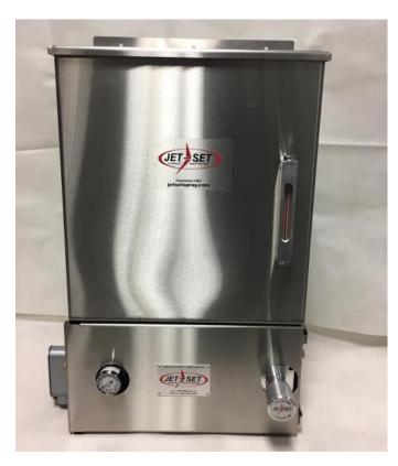
The MOD-1E JET-SET® spray system comes standard with our 10 Gallon stainless steel tank with sight gauge, reusable filter, and air regulator. This system includes one JET-SET 9100 stainless steel piston pump (0-5cc per stroke) with 5 outlets for spray nozzles. The 9100 pump is engaged using the electric solenoid to receive external signals for system activation. The MOD-1E comes standard 110v unless specified.
