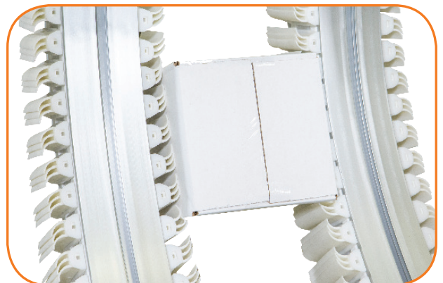
Products are wedged between opposing conveyors
