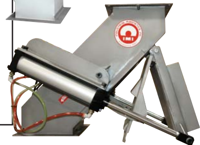
Single Leg Hump Magnet (Air-Actuated Self-Clean Shown)
