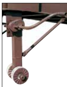
MANUAL HAND CRANK AND 8-5/8" STEEL WHEELS
