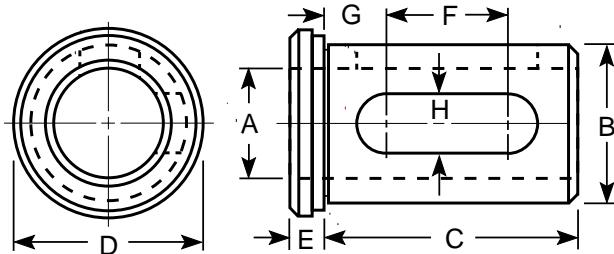
Acme Type C Tool Holder Bushings have an elongated slot to allow set screws to properly clamp on the shank of tools. Type C bushings are hardened and ground for a more accurate, longer lasting bushing.
