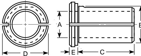
Type B Tool Holder Bushings are split through the entire length of the bushing on one side. This enables the bushing to clamp on the shank of cutting tools by tightening the screws in the turret bore or tool holder. Acme Type B bushings are hardened and precision ground to provide a longer lasting more accurate bushing. Solid, soft blanks with a machine finish are available upon request.
