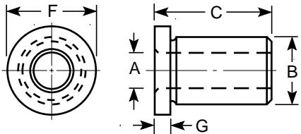
Head Liners are dimensionally the same as Head Press Fit Bushings so they both have the same type designation "HM". Some catalogs may refer to Head Liners as type "HLM". Please note that the length on type "HM" bushings and liners is measured overall.
