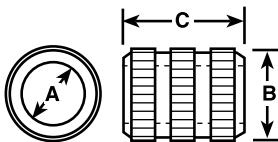
The Ser-Groove (SG) bushing consists of a serration that permits the bushing to be pressed into a jig or fixture made of soft material or laminated fiberglass while maintaining its holding strength.
