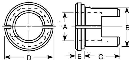
Acme Tap Holder Bushings are split along the body with a square recess milled in the back to firmly grip and drive taps. Tap holder bushings are left soft to protect the tap. Type K bushings are precision ground for proper alignment.
