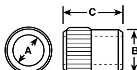
The Spline-Lock (SL) type bushing features a partially serrated and partially ground outside diameter. This configuration enables the bushing to be pressed into soft metals or wood.
