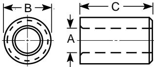
Extended Range Bushings with a ground O.D. are concentric within .0005" T.I.R. Unground Extended Range Bushings have a concentricity of .006" T.I.R. To order an unground O.D., add the letter "U" to the end of the ANSI designation.
