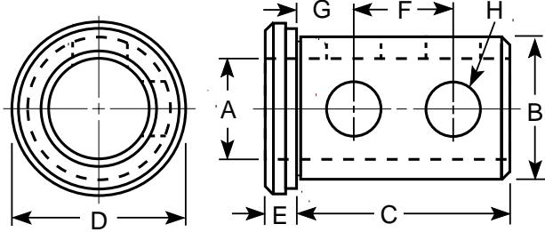
Acme Type J Tool Holder Bushings have clearance holes for set screws for proper clamping on the shank of tools. These bushings are hardened and ground for long life and accurate alignment. Solid, soft blanks for custom machining are available on request.
