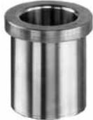
All Head Liners are honed or ground in the I.D. and are concentric within .012 T.I.R. to the O.D.
