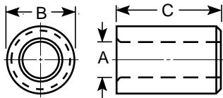
All liner bushings are honed or ground in the I.D. Liners with I.D.'s 3/16" to 1" are concentric within .0003" T.I.R. to the O.D. Other I.D. sizes are held within .0005" T.I.R. All unground bushings are left rough on the O.D. with concentricity of approximately .006" T.I.R.
