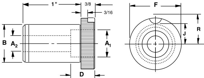
Acme Gun Drill Liners are designed to be used with the replaceable inserts indicated in the table below. All type GDL Bushings are ground concentric within .0002" T.I.R. The heads are undercut and ground square with outside diameters so the liner will seat flat against the chip box.
