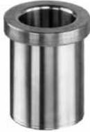
All press fit bushings are lapped, honed or ground in the I.D. and are concentric within .012 T.I.R. to the O.D.
