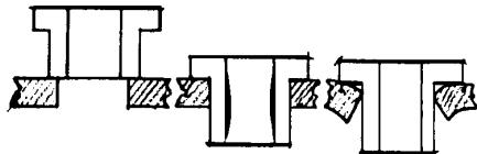
Too little interference may allow slippage, thus causing inaccurately drilled holes. In most cases, interference of 0.0005 to 0.0008 inch is sufficient to properly install press fit bushings and liners.
