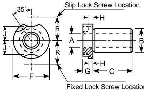
Extended Range Slip-Fixed Renewable Bushings are ground to slip fit into Liners and are concentric within .0005" T.I.R.
