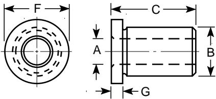
Extended Range Bushings with a ground O.D. are concentric within .0005" T.I.R. Unground Extended Range Bushings have a concentricity of .006" T.I.R. To order an unground O.D., add the letter "U" to the end of the ANSI designation.
