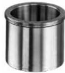
All liner bushings are honed or ground in the I.D. Liners with I.D.'s 3/16" to 1" are concentric within .0003" T.I.R. to the O.D. Other I.D. sizes are held within .0005" T.I.R. All unground bushings are left rough on the O.D. with concentricity of approximately .006" T.I.R.
