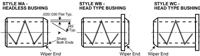
**Wiper Specifications:** Oil groove does not run out on wiper end.
