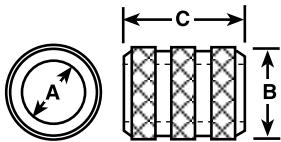
The Diamond-Groove type (DG) has a special knurl that provides superior holding strength in potting compounds and castable materials. The number of grooves is dependent on the length of the bushing.
