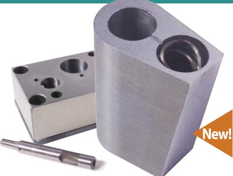
Dayton EZ Fit<sup>™</sup> Ball Lock Retainer Inserts give you the ability to reconfigure and custom-make retainers inhouse as die specifications change. The unique singlepiece teardrop shape, combined with both a straight and an angled wedge side, holds your ball lock punch securely in place. EZ Fit<sup>™</sup> Inserts reduce costs and downtime—and simplify tooling changeover.
