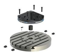
Mount direct to t-slotted machine table. Locate with center pin and timing key. Secure to table with t-nuts & SHCS
