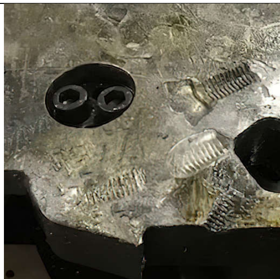
Competitor's vulnerable design allows screws to loosen and fall into the die, damaging product and other tooling.
