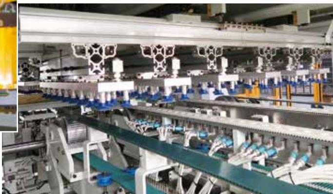
Cup feeder and vacuum conveyor for aluminum transfer
