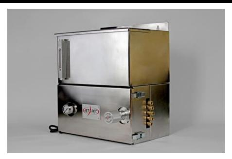
The MOD-1E JET-SET® spray system comes standard with our 5 Gallon stainless steel tank with sight gauge, reusable filter, and air regulator. This system includes one JET-SET 9100 stainless steel piston pump (0-5cc per stroke) with 5 outlets for spray nozzles. The 9100 pump is engaged using the electric solenoid to receive external signals for system activation. The MOD-1E comes standard 110v unless specified.
