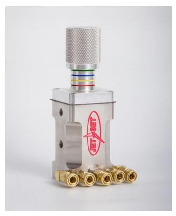
All JET-SET® Module Systems have the new stainless steel JET-SET® pump designed for long life cycles. Utilizing stainless components and viton seal. The #9100 pump will give millions of cycles of maintenance-free operation. All JET-SET® pumps provide easy volume regulation by turning the large knob on top of the pump. You can regulate the output of fluid from 0 to 5 cc per cycle. One to three pumps may be mounted in the system. All pumps have five quick disconnect fittings for nozzles.
